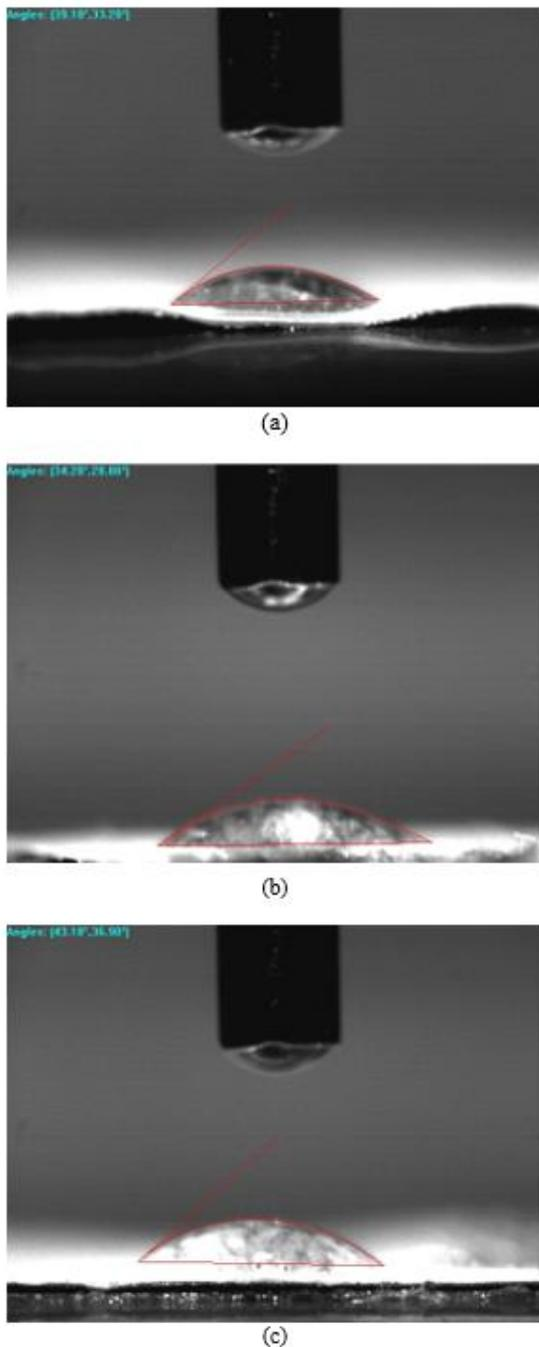
**Fig 2** Water contact angles of electrospun PVA nanofiber membranes: (a) PVA1, (b) PVA2 and (c) PVA3.
