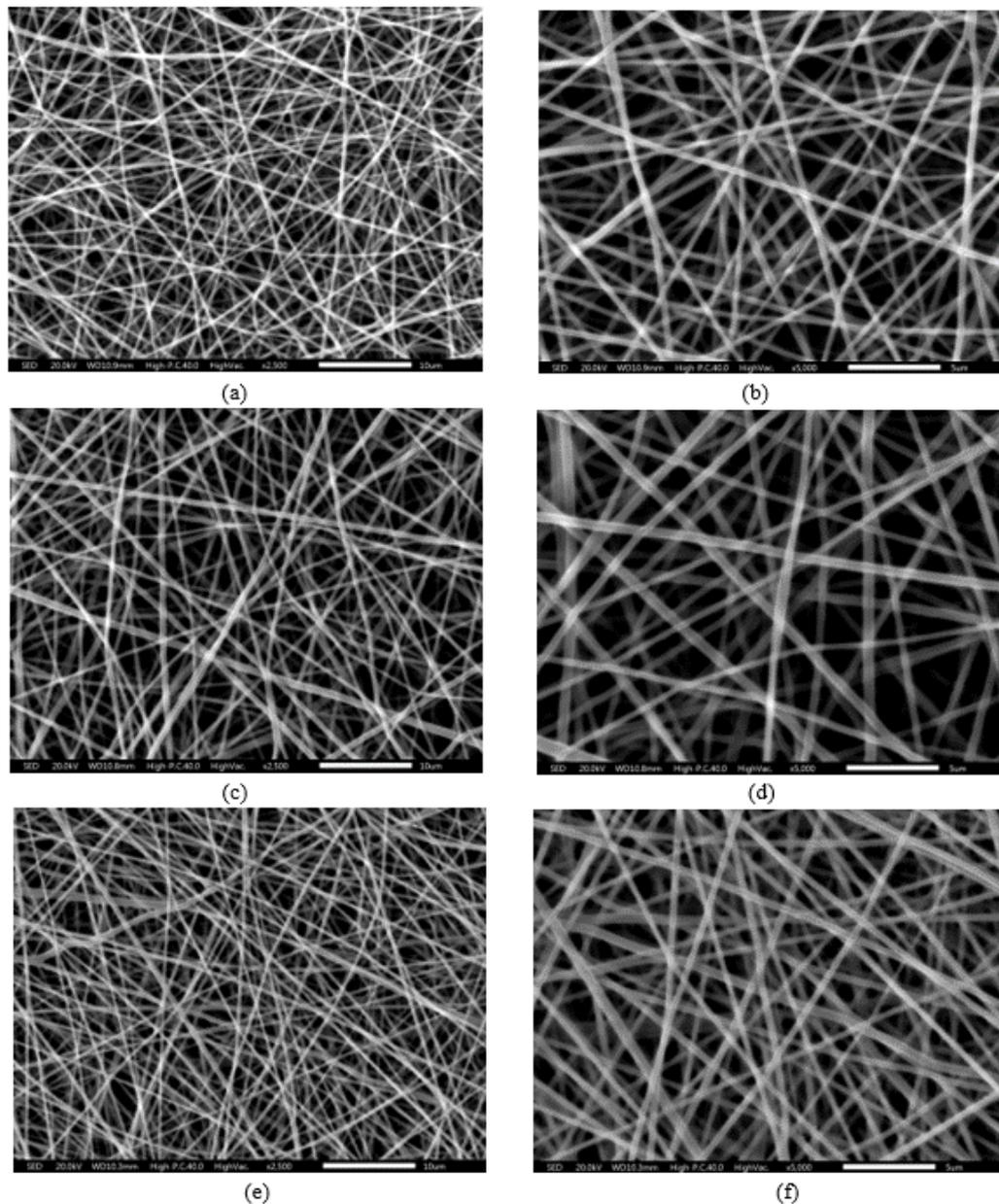
**Fig 1** SEM micrographs of electrospun PVA nanofiber membranes at 2,500x and 5,000x magnifications for samples (a,b) PVA1, (c,d) PVA2 and (e,f) PVA3.
