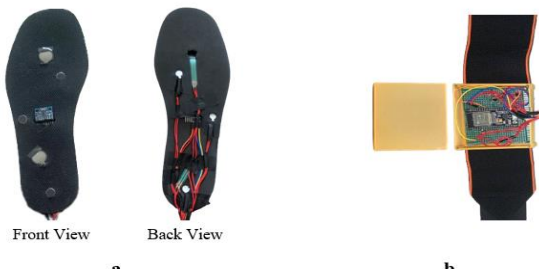
Fig. 7 (a) Front and back view of the middle layer, (b) 3D printed box and PCB circuit board
