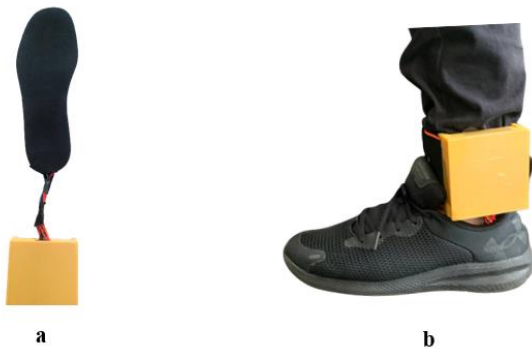
Fig. 8 (a) Complete smart insole prototype, (b) Device placed on human leg
