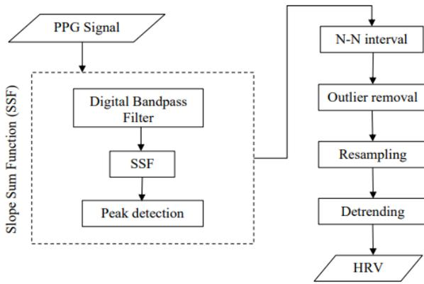
Fig. 2 Signal preprocessing algorithm.
