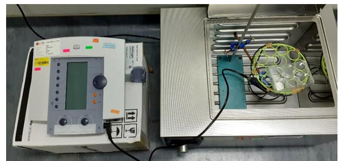
Fig. 2 The setup of the ultrasound transducer in a water bath.
