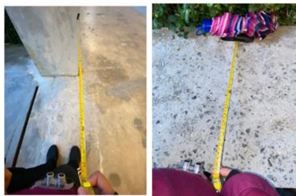
Fig. 2 The setting sample process for the sensor detection test at 50 cm (a) indoor and (b) outdoor
