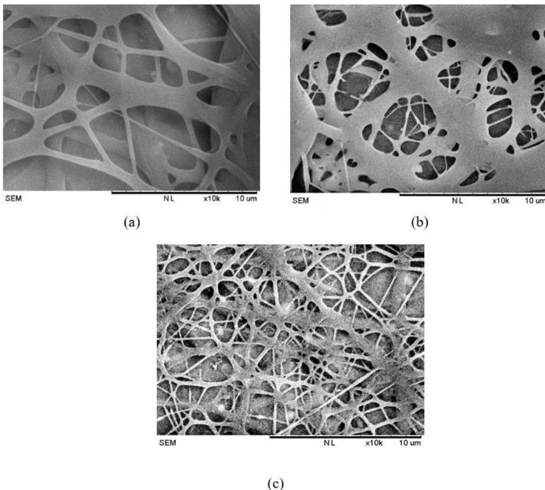
**Fig 1** SEM image of nanofibers for (a) PCL, (b) PCL/Gelatin (60:40) (c) PCL/Gelatin (70:30)
