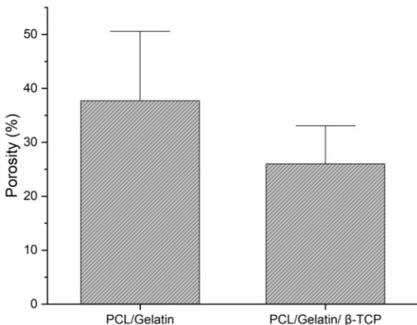
**Fig 3** Porosity of PCL/Gelatin and PCL/Gelatin/ $\beta$ -TCP nanofiber at 70:30 (PCL: Gelatin) ratio.
