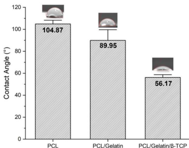
**Fig 5** Contact angle measurement for PCL, PCL/Gelatin and PCL/Gelatin/ $\beta$ -TCP. Data shown as mean  $\pm$  standard deviation with  $n = 3$ .
