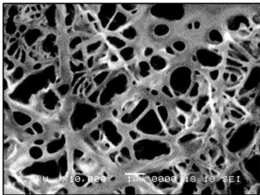
**Fig 2** SEM image of PCL/Gelatin/ $\beta$ -TCP nanofibers at 70:30 (PCL: Gelatin) ratio
