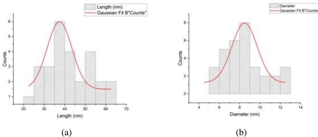
Fig. 4 (a)Gaussian distribution on HA nanoparticles length (b)Gaussian distribution on HA nanoparticles diameter
