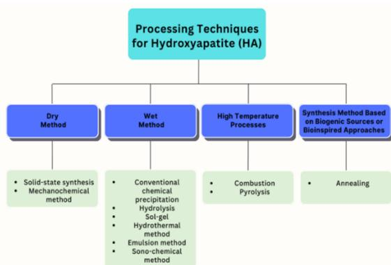
**Fig.1** Processing techniques for hydroxyapatite
