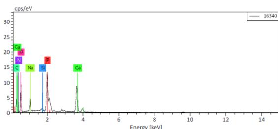
**Fig. 5** EDX spectra of hydroxyapatite nanoparticles
