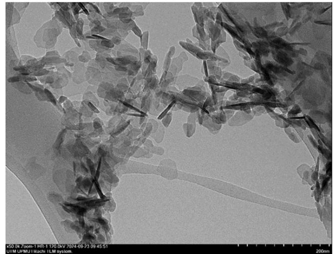
Fig. 3 TEM micrographs of hydroxyapatite nanoparticles
