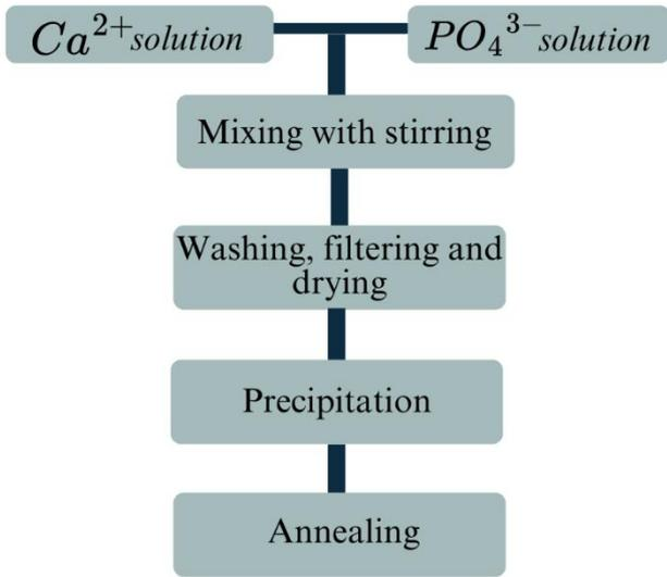
Fig. 2 Co-precipitation procedure
