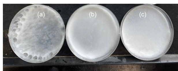
Fig 1 Gelling time took by the samples to become hydrogel (a) PVA/pectin hydrogel (1 hour), (b) PVA/pectin hydrogel with 5% hydroxyapatite (1.5 hours) and (c) PVA/pectin hydrogel with 10% hydroxyapatite (2 hours)
